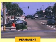
"Curb Extensions" are most often used at pedestrian crossings, where the extension of the curb into the roadway narrows the distance between curbs and improves the pedestrian environment.
