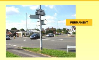
These smaller versions of regular traffic circles are designed for narrower residential streets. The center island is usually painted and slightly domed. Larger vehicles can drive over the edges of it. Where space permits, small islands on each approach deflect traffic away from a straight path. All entering traffic yields to the left. Traffic circles reduce travel speeds.
